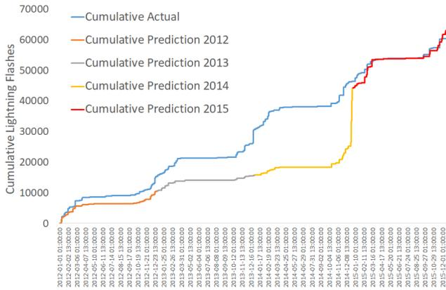
Fig. 2. Cumulative Actual vs Cumulative Predicted 1HR Lightning Flashes for Bloemfontein between 2012 to 2015..
