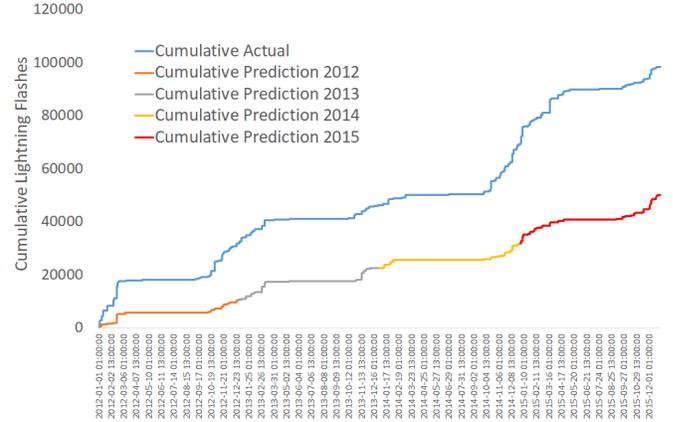
Fig. 1. Cumulative Actual vs Cumulative Predicted 1HR Lightning Flashes for Piet Retief between 2012 to 2015.
